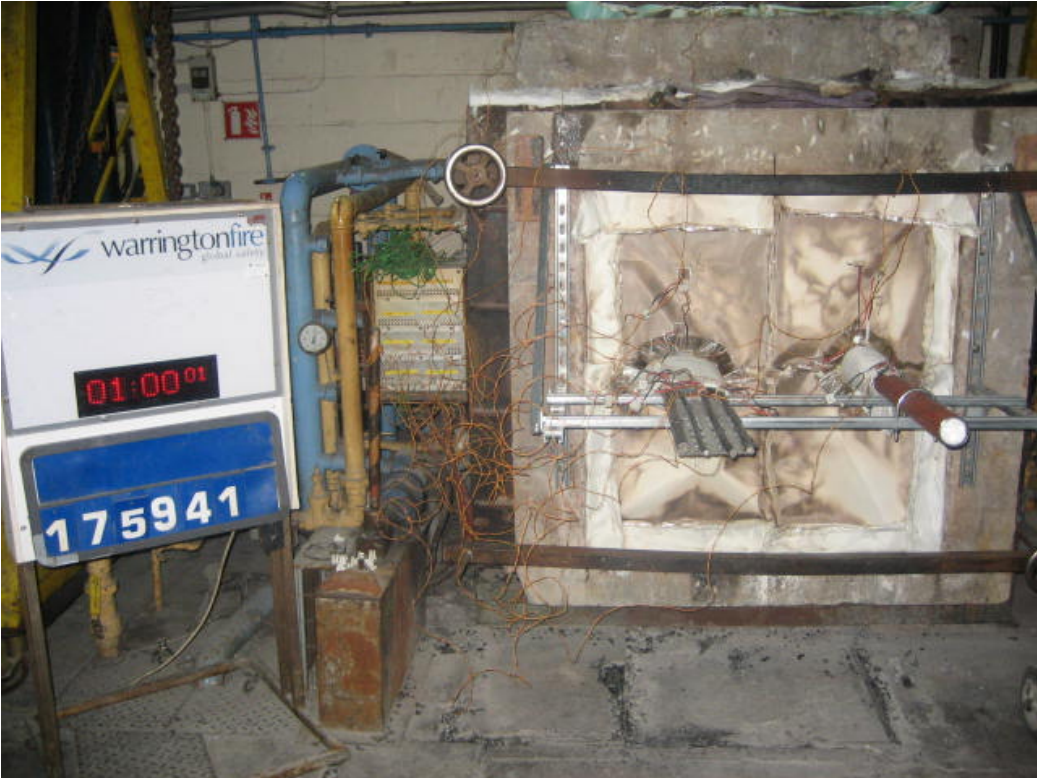
The unexposed face of the seals after a duration of 60 minutes
