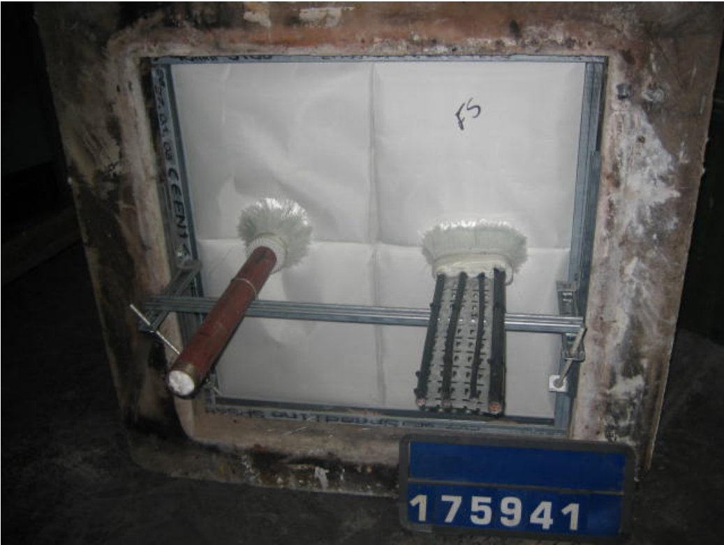
The exposed face of the seals prior to testing
